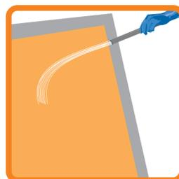
Apply XMP- Heavy Duty Mesh Prep to both sides of the screen and rinse off with a garden hose.
