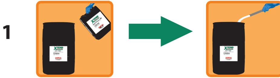
**1** Add 2 gallons of XSR-155 stencil remover to a drum of XID-480/25 ink degradable and then fill the remainder of the drum with water.
