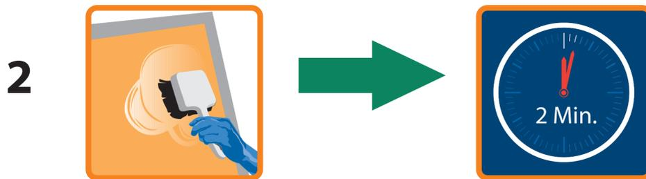
**2** Apply mixed solution using a brush or spray to both sides of a screen that has had the ink scraped out. Leave for 2 minutes.
