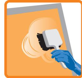
Apply XHR-AN using a brush to both sides of a screen. Leave about a 10" gap from the edge of the frame.
